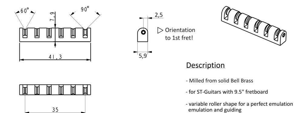
fills the widened gap that has to be made in order to place the rollers in the middle of the point support of the former non-roller saddle
