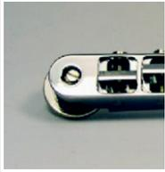
*Our milled string-saddle has got precise defined edges and flanks. The saddle-shoulder presents full contact to the bridge. No rattle of the spring occurs due the intonation-screw is anchored by a circlip! An ABM T.O.M-Bridge offers 0,8 to 1,3mm more intonation-range than the actual original ABR-1 and Nashville bridge features.*
