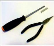
**Tools:** Slotted screwdriver (S = 1,0mm), a piece of rubber hose (makes the work safe & easy, with a 4,5mm bore diameter) and fine long-nose-pliers.
