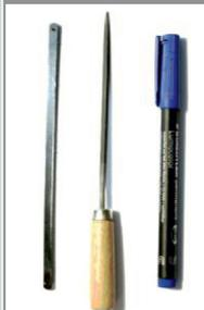
A round „U-Groove“ may be the best notch-type, but you need several files following the exact string gauges. Buzzing noise may occur when a string does not complete the notch („Sitar-Effect“). Notches wear out and the problem will occur some day in either case. We prefer „V-Cut“-Notches with their long lasting fit and best tone transmission too.
