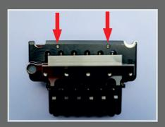
For this purpose, the screws have a conical tip which lateral surface presses the knife edge into the slot when the screw is screwed in.
