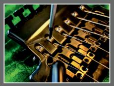
2. Then please review whether the two saddle lock screws attached to the side of the tremolo base plate are tight. These prevent movement of the saddles.
